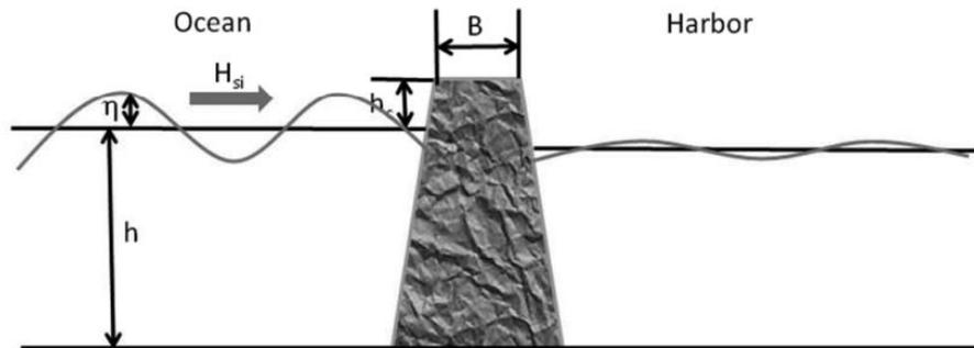
Figure 8-6: Conceptual Sketch of Wave Transmission through a Breakwater (Li et al. 2011)
